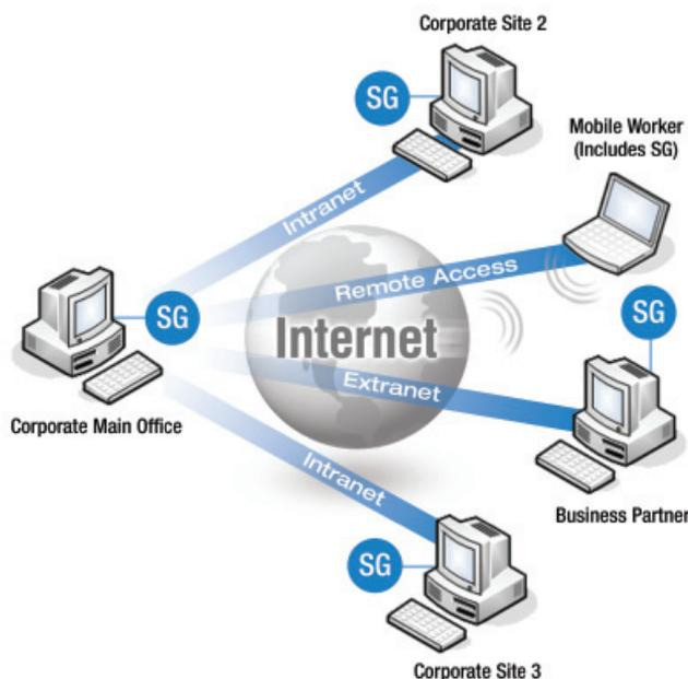
*IPsec ensures secure data transmission when using the public Internet as a VPN backbone.*
