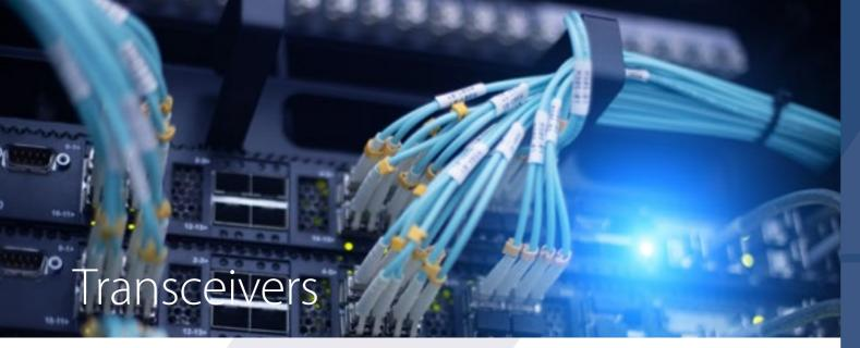
Transceivers allow for the expansion of Ethernet networks by providing high-speed connections over a fibre-optic cabling. The fibre-optic transceivers have standard duplex LC connectors to provide maximum compatibility. They are hot-pluggable and Small Form Factor Pluggable (SFP) compliant with the Multi-Source Agreement (MSA) specification.
