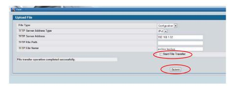
6. Once the transfer is complete you can find the backup file in the installation path of the TFTP server
