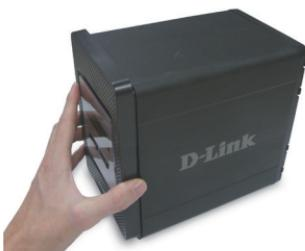
2. Once the faceplate is unlatched, pull it off of the device, exposing the drive bays.
