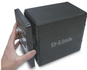
3. Insert a 3.5" SATA hard drive into an available drive bay. Make sure to align the drive connector to the endpoint in the DNS-343. Gently push the drive in until it connects. Repeat for each drive you are placing in the DNS-343.
