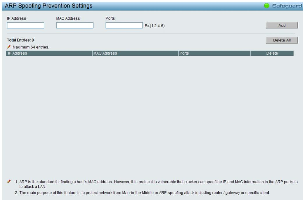
Figure 5.86 – Security > ARP Spoofing Prevention Setting
