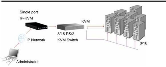
Figure 3-1.b: IP-KVM switch usage scenario
