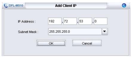
3. Type in the IP Address and Subnet Mask for the PC that will access the DFL-M510 and click **OK**. The IP Address is added to the Selected IP Address window. Repeat steps 2 and 3 to add other IP Addresses.
