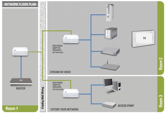
\*A minimum of two D-Link PowerLine HD Network Adapters are required to create a network.
