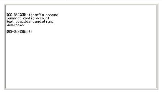
Figure 2-3. Example Command Parameter Help
