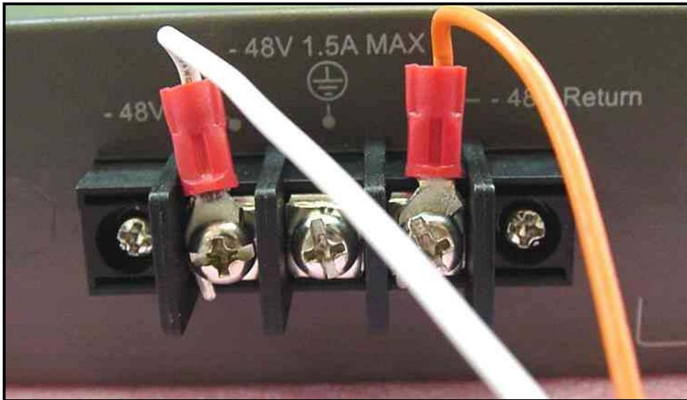
**Figure 2- 7. Power connections attached to contacts on assembly**
