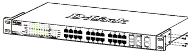
Figure 2. Attaching the mounting brackets
