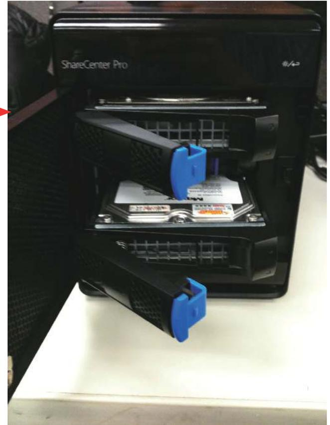
**Step 5:** As you install the second drive, the ShareCenter Pro automatically recognizes the drives and displays the information on the OLED screens.
