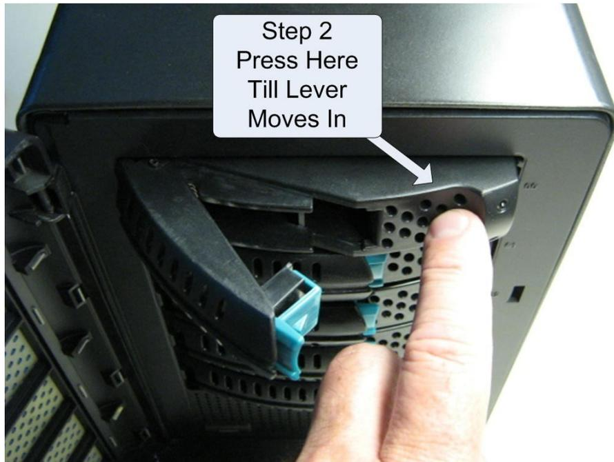
Figure A-22 Press Here Until You See the Lever Move Inwards
