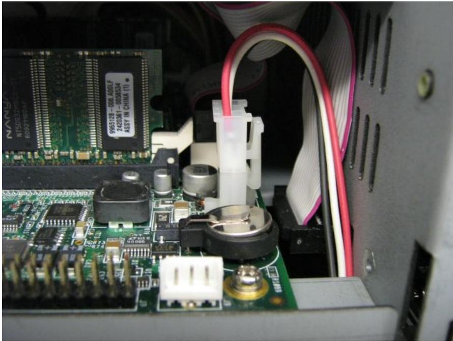
**Figure A-8 Battery Plug Locked in Place**
