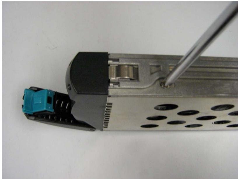
**Figure A-20 Secure the Hard Drive in the Drive Tray**
