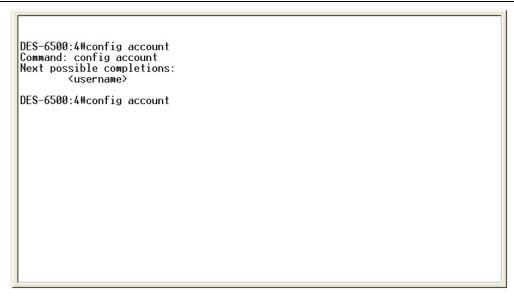
Figure 2-3. Example Command Parameter Help
