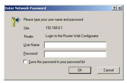
In order to configure the Broadband Router you must input the user-name into the **User Name** box. Enter the password into the **Password** box and press the **OK** button. The default User Name is "Admin". There is no default password, leave the Password field blank.
