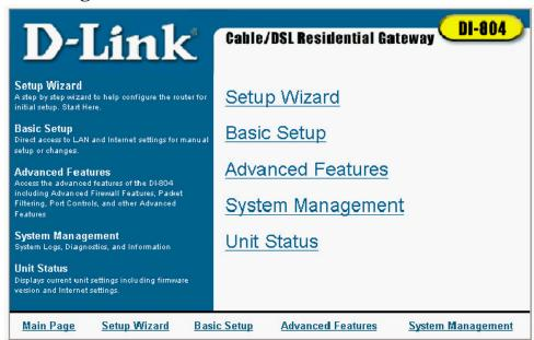
The Main Page screen provides links to the main sections of the web configuration interface. Each section is described in detail in the following sections of this manual. The Unit Status links to the status screen to view current status of your internet connection and is described in the System Management chapter.
