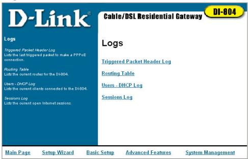
The Logs screen can be used to display information logs pertaining to different aspects of your DI-804. Clicking on the links will display a pop-up screen containing the desired information.
