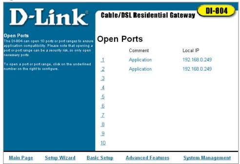
The DI-804 can open ports or port ranges to ensure application compatibility. This screen shows which Open Ports rules you have configured. Please note that opening a port or port range can be a security risk, so only open necessary ports.
