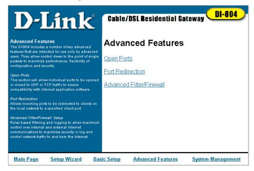
**Open Ports**: Allows specific ports to be opened to allow certain Internet applications to work correctly.
