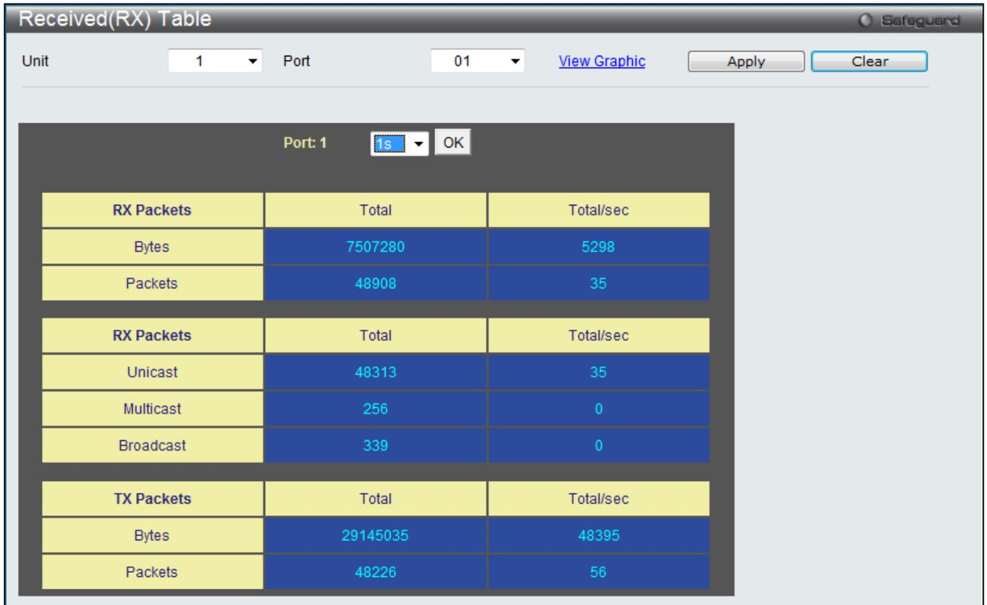
Figure 11-5 Received (RX) Table window (for Bytes and Packets)
