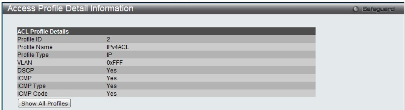
**Figure 7-9 Access Profile Detail Information window (IPv4 ACL)**
