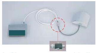
Install the surge protector as recommended position when you do not purchase the low loss cables (ANT24-CB03N, ANT24-CB06N and ANT24-09N...)
