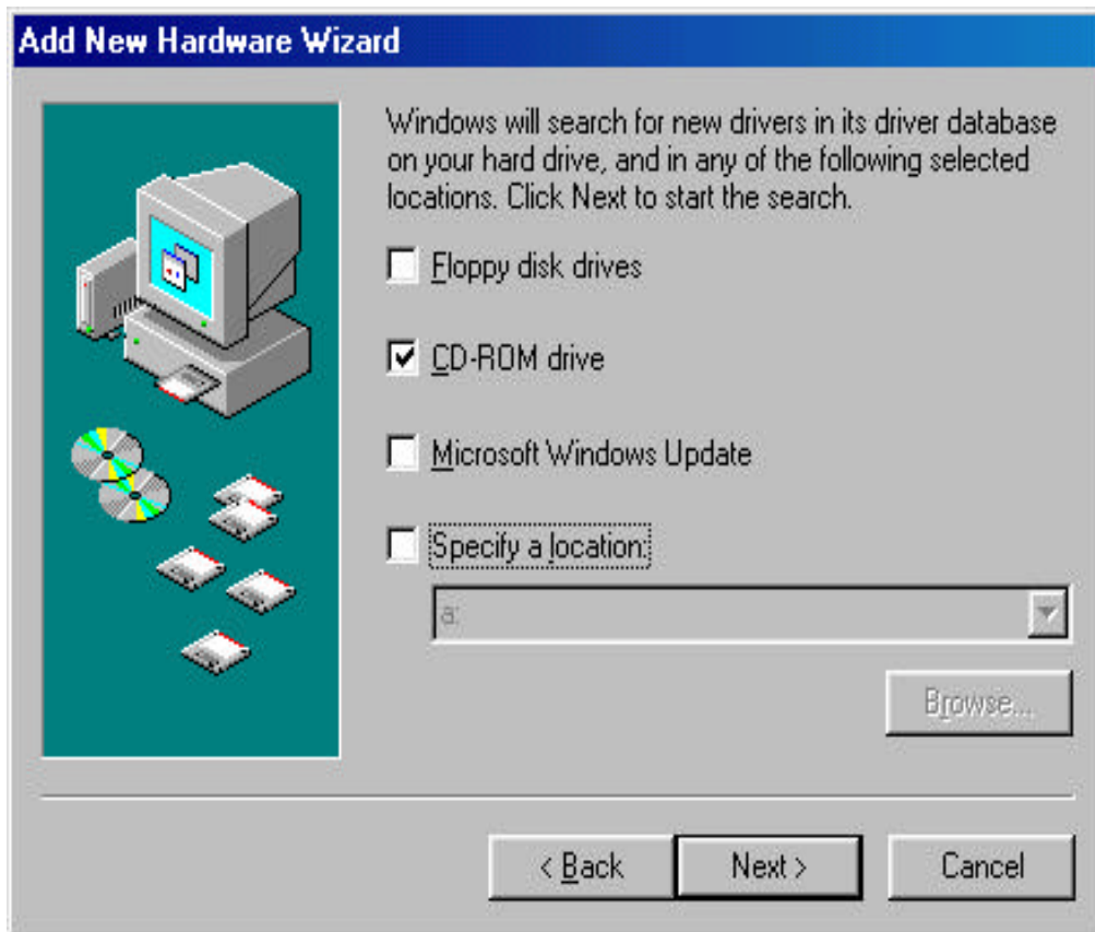
Figure3- Enter CD-ROM drive, or click on the Browse button and select CD-ROM drive.
