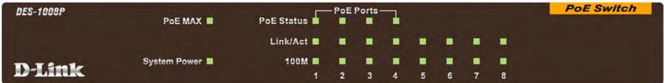
**Figure 3. LED indicators of the Switch**
