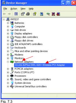
Look under Device **Status** to check that the device is working properly.
