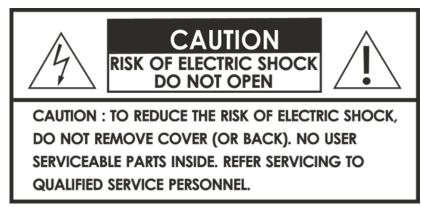
The lightning flash with arrowhead symbol, within an equilateral triangle, is intended to alert users to the presence of uninsulated "dangerous voltage" within the product's enclosure that may be of sufficient magnitude to constitute a risk of electric shock to persons.
