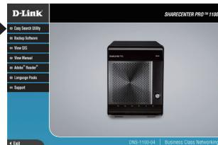
Select the listed ShareCenter Pro and click the Configuration button. This will launch the computer's default web browser and direct it to the IP address listed for the device. Make sure the browser is not configured to use a proxy server.
