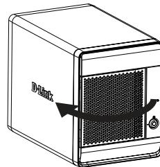
2. Remove the HDD tray by pressing the green button.
