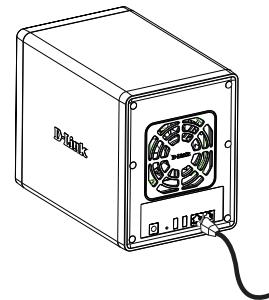
6. Connect the supplied power adapter to the power receptacle.
