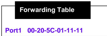
In addition, when the Switch receives the broadcast ARP request, it will flood the frame to all ports except the source port, port 1 (see Figure -2).
