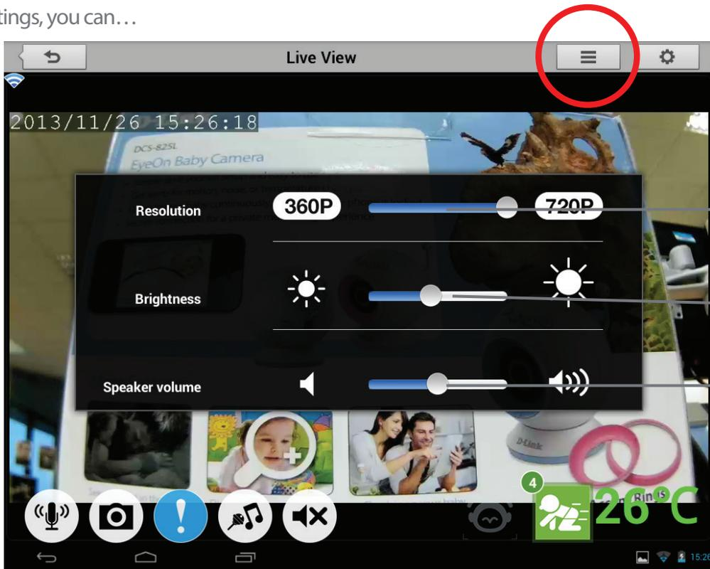
Change your EyeOn Baby Camera resolution between 360P and 720P. 360P resolution will give you a faster response, whereas the 720P resolution will give you a higher resolution image.
