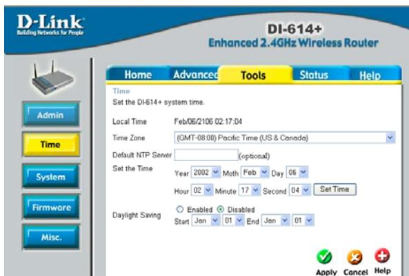
The screenshot shows the 'Tools' section of the D-Link DI-614+ web interface. The 'Time' tab is selected. The page title is 'DI-614+ Enhanced 2.4GHz Wireless Router'. The navigation menu includes Home, Advanced, Tools, Status, and Help. The 'Time' section contains the following fields and options:
