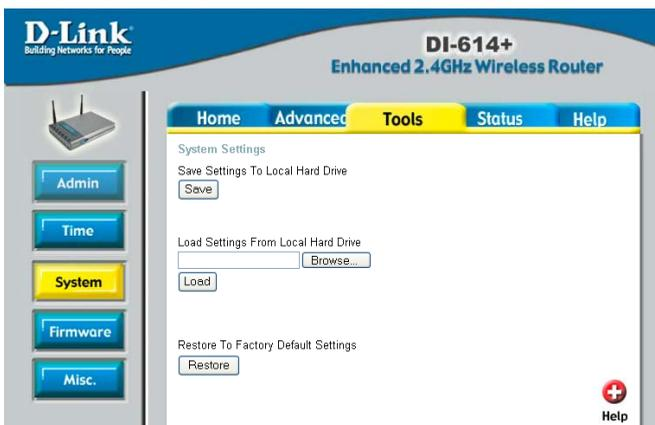
The screenshot shows the 'System Settings' page in the 'Tools' section of the D-Link DI-614+ web interface. The page title is 'DI-614+ Enhanced 2.4GHz Wireless Router'. The navigation menu includes Home, Advanced, Tools, Status, and Help. The 'System Settings' section contains the following options:
