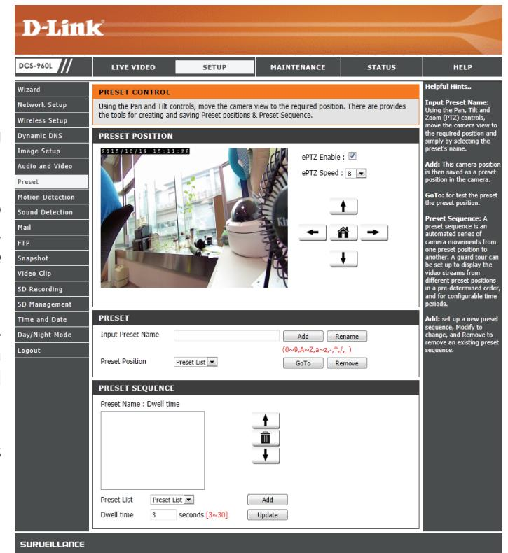
**Preset List:** To add a preset to the sequence, select it from the drop-down box at the bottom of this window, set the Dwell time to determine how long the camera view will stay at that preset, then click the **Add** button. The preset name will appear in the list, followed by the dwell time to view that preset for.
