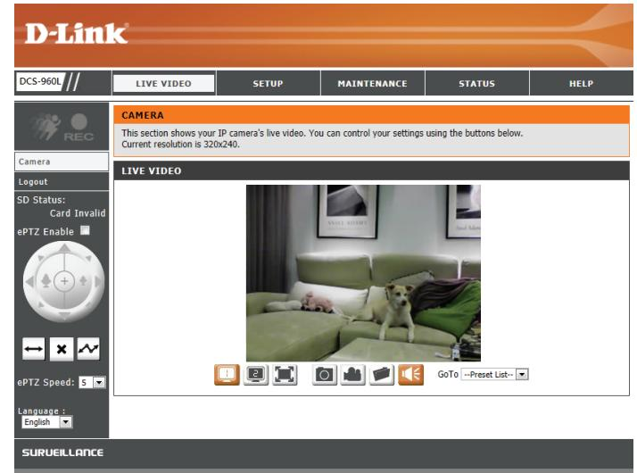
**ePTZ Enable:** Checking this box will allow you to use ePTZ, which will give you a zoomed view of the camera's Live Video that you can use the control pad to move around.
