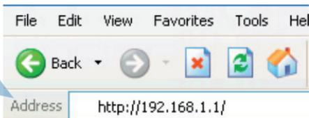
(The IP Address shown in the example above is the default setting. If you have changed the IP Address of the DFL-800 to conform to a network, then input that IP Address in the web browser, instead of the default IP Address shown.)
