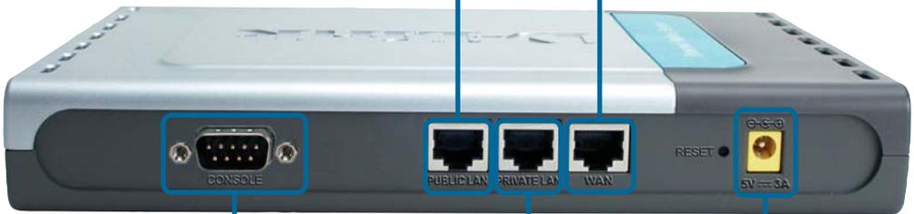
**CONSOLE:** Connects to your computer's COM port using the provided Console Cable. (Port also connects to optional DSA-3100P Ticket Printer)
