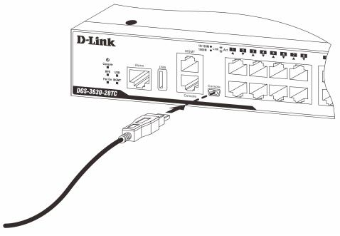
Figure 5-2 Connect Mini-USB Console Port
