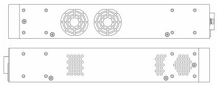
Figure 2-4 Side panels of the DGS-3630-28TC
