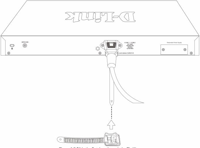
Figure 3-7 Slide the Retainer through the Tie Wrap
