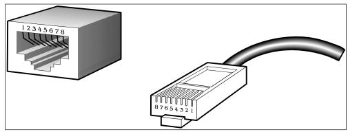
Figure B-1 Standard RJ45 port and connector
