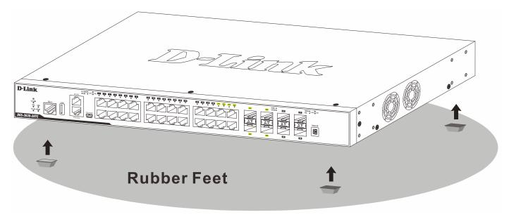
Figure 3-1 Attaching rubber feet to the Switch
