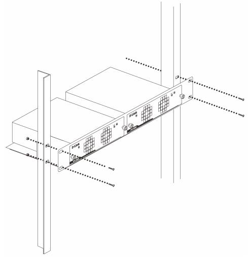
Figure 3–12 Install the DPS-800 in an Equipment Rack
