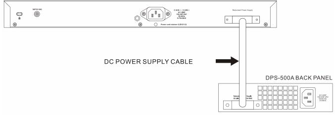
Figure 3–10 Connecting a DGS-3630 Series Switch to the DPS-500A
