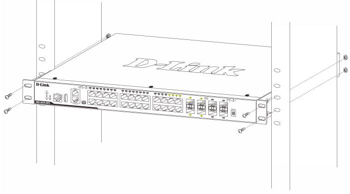
Figure 3-3 Installing the Switch in a Rack
