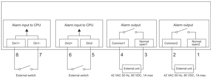
Figure B-5 Alarm Connector pinout
