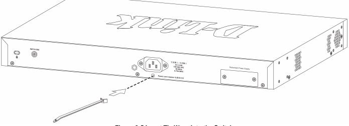
Figure 3-5 Insert Tie Wrap into the Switch
