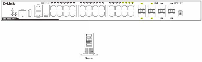
Figure 4-5 Connecting the Switch to a server
