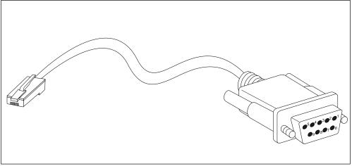
Figure B-2 Console to RJ45 Cable
