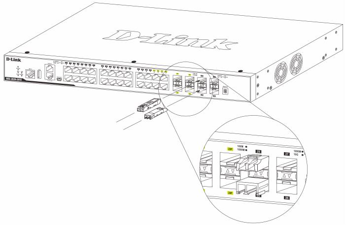
Figure 3-4 Inserting transceivers into the transceiver ports
