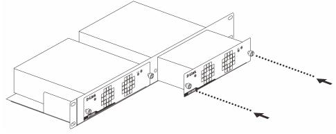
Figure 3–11 Install the DPS-500A in the DPS-800
