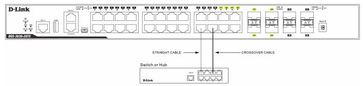
Figure 4-2 Connecting the Switch to another switch/hub
