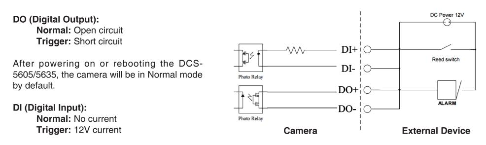
As the Digital Input signal is controlled by an external device, we recommend that you set your device to feed no current normally, and feed a 12V current only to trigger a DI event on the DCS-5605/5635.
