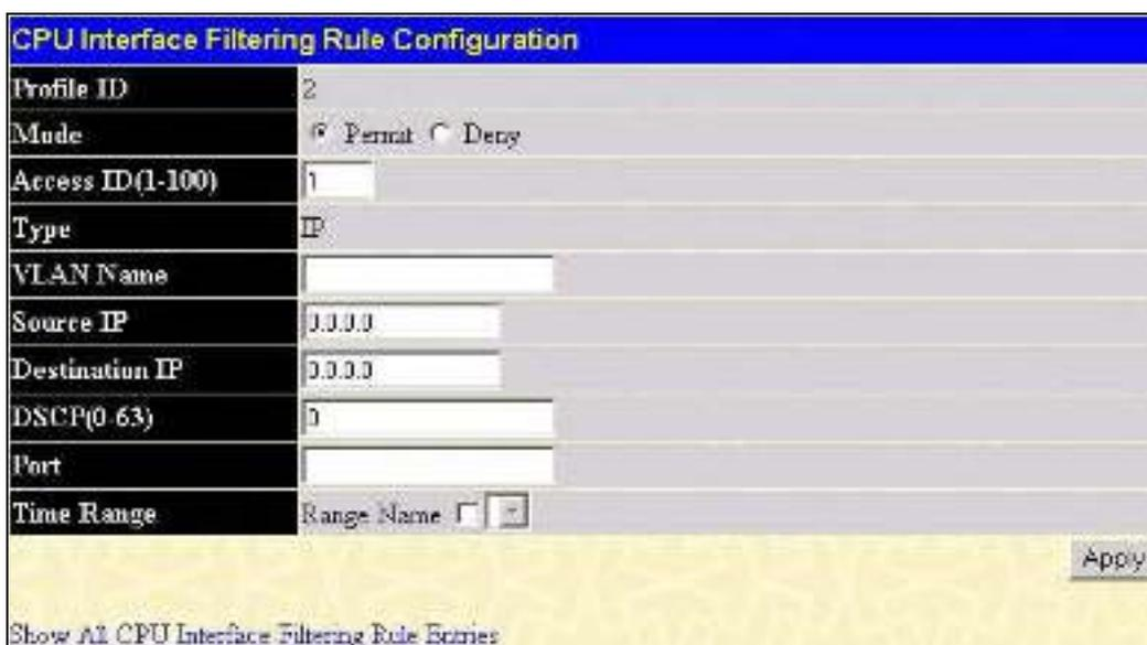
**Figure 10- 34. CPU Interface Filtering Rule Configuration window (IP)**
