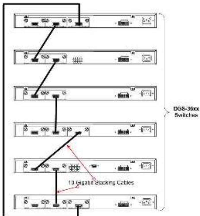
Figure 6- 3. Switches stacked in a Duplex Ring
