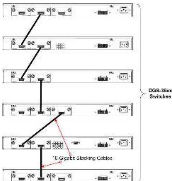
Figure 6- 2. Switches stacked in a Duplex Chain
