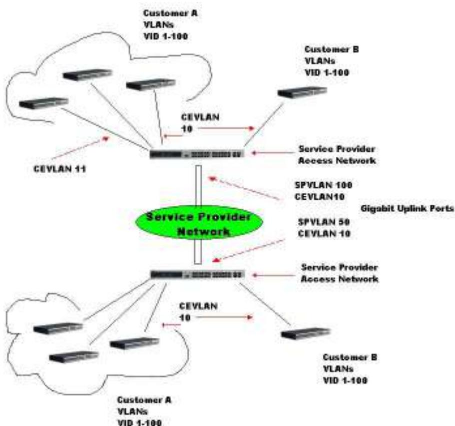
**Figure 7- 9. Double VLAN Example**
