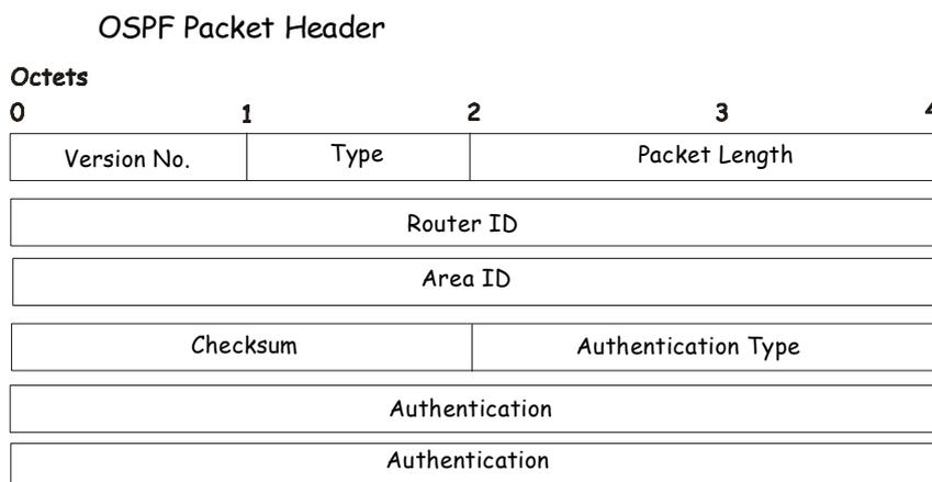
**Figure 8- 25. OSPF Packet Header Format**
