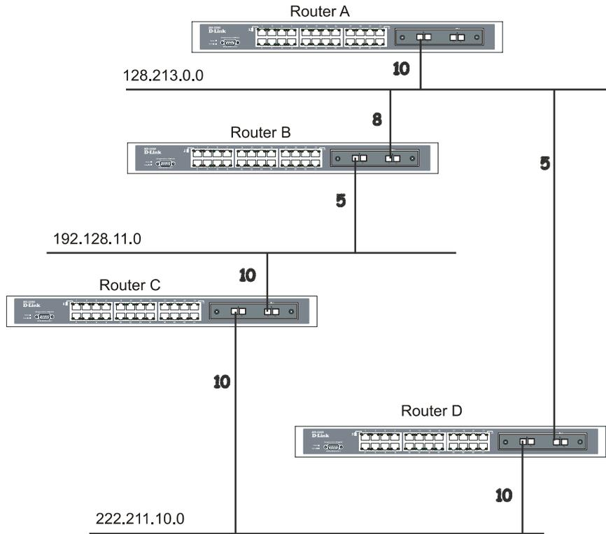
Figure 8- 22. Constructing a Shortest Path Tree
