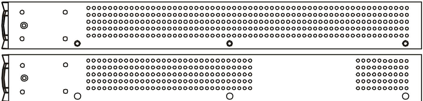
Figure 1- 13. Side Panels of the DGS-3650
