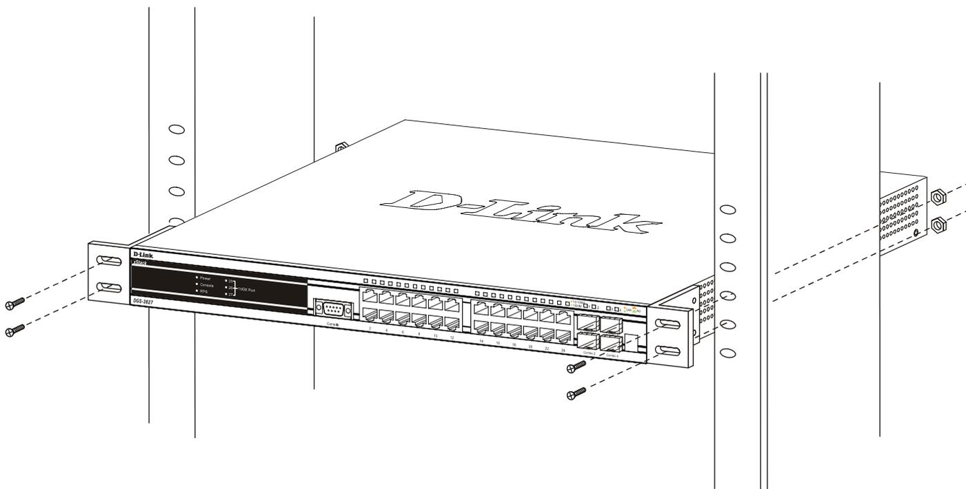
Figure 2 - 3. Installing Switch in a rack
