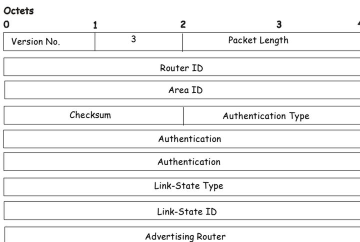
Figure 8- 28. Link-State Request Packet
