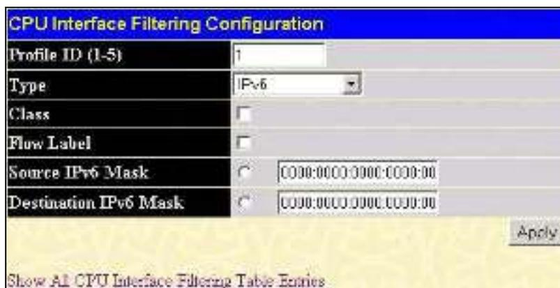
**Figure 6- 82. CPU Interface Filtering Configuration window (IPv6)**
