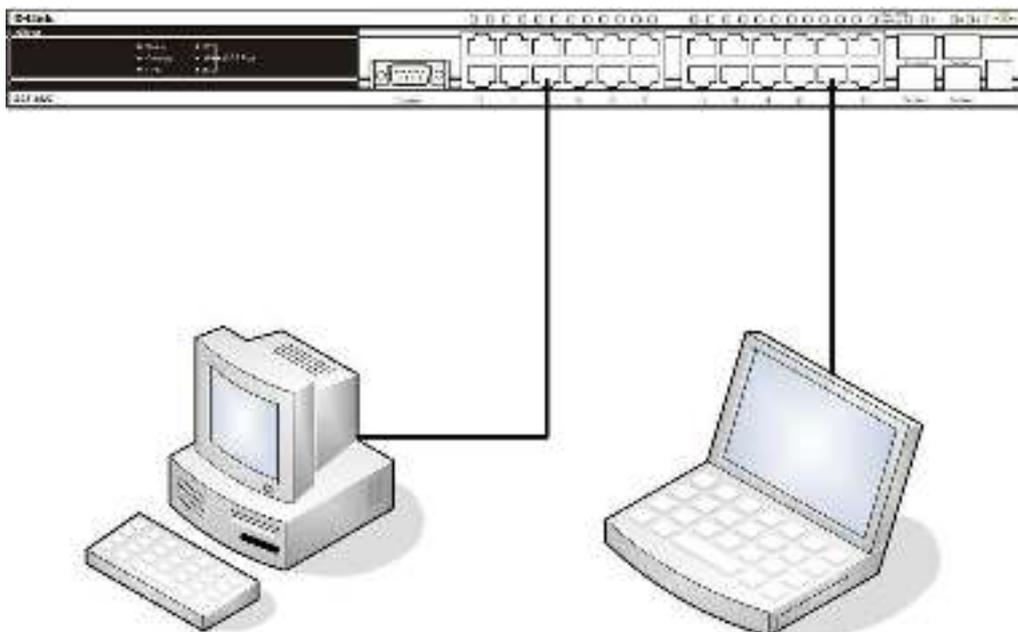
**Figure 3- 1. Switch connected to an end node**
