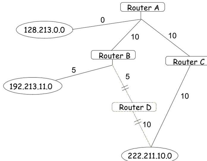
Figure 8- 23. Constructing a Shortest Path Tree
