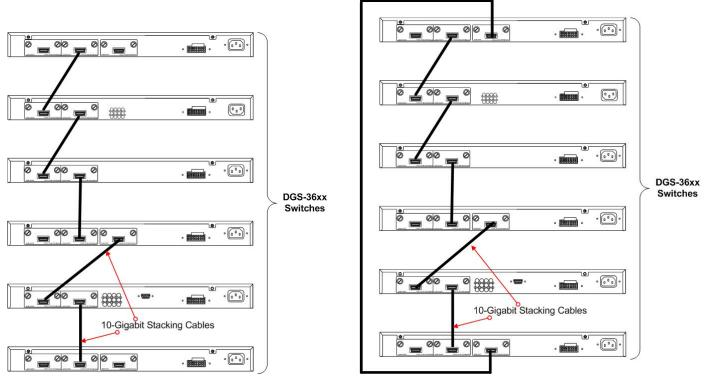
Figure 2-4. Switches stacked in a Duplex Chain
