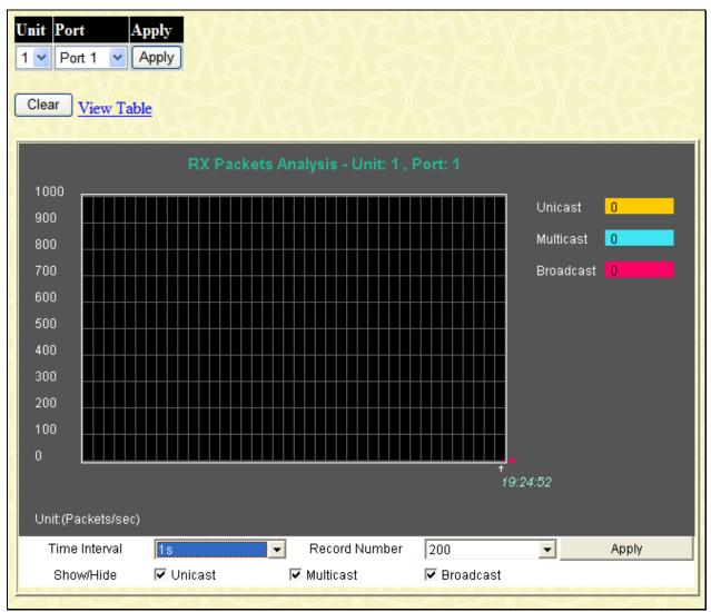
**Figure 8- 10. RX Packets Analysis window (line graph for Unicast, Multicast, and Broadcast Packets)** To view the UMB Cast Table, click the <u>View Table</u> link, which will show the following table:
