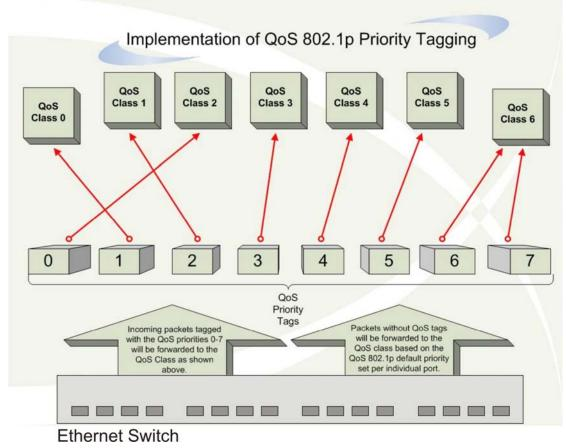
Figure 5-1. Mapping QoS on the Switch
