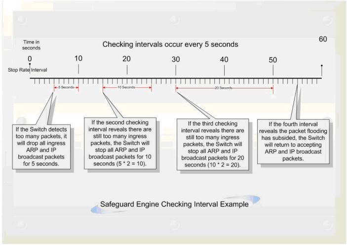
Figure 7-61. Safeguard Engine example
