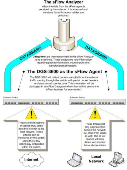
Figure 2-81. sFlow Basic Setup
