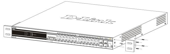
Figure 2 - 2. Fasten mounting brackets to Switch
