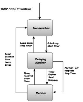
Figure 8-71. IGMP State Transitions
