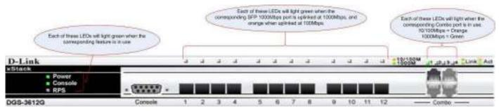
Figure 1- 5. DGS-3612G LEDs
