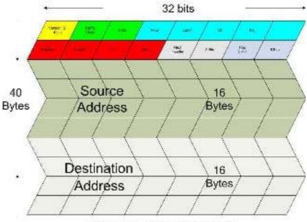
Standard IPv6 Packet Header
