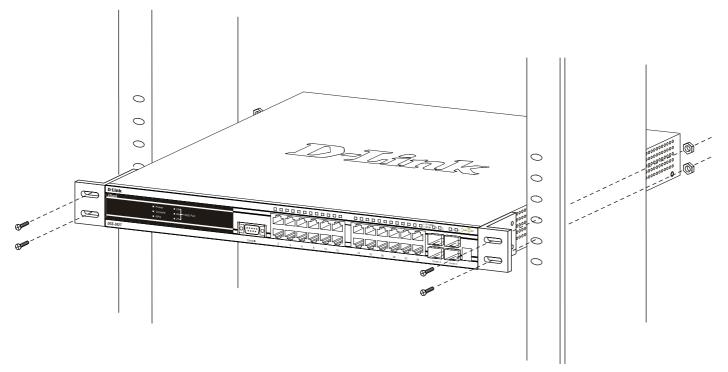
Figure 2 - 3. Installing Switch in a rack
