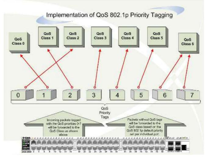
Figure 9-1. Mapping QoS on the Switch
