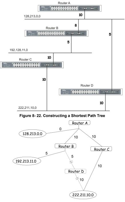
Figure 8-23. Constructing a Shortest Path Tree
