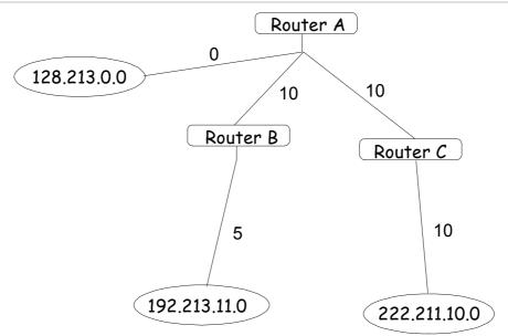
Figure 8-24. Constructing a Shortest Path Tree - Completed
