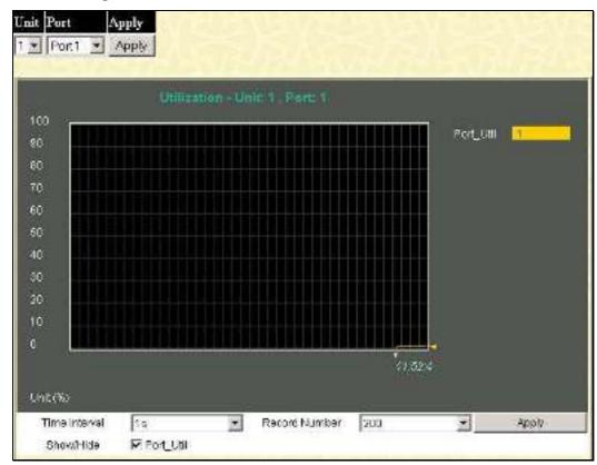
Figure 12- 5. Port Utilization window
