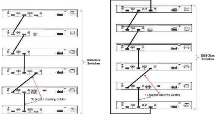
Figure 6-2. Switches stacked in a Duplex Chain
