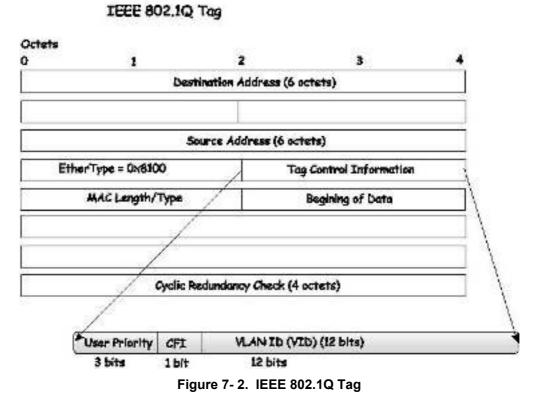
The EtherType and VLAN ID are inserted after the MAC source address, but before the original EtherType/Length or Logical Link Control. Because the packet is now a bit longer than it was originally, the Cyclic Redundancy Check (CRC) must be recalculated.
