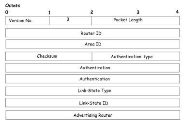
Figure 8- 28. Link-State Request Packet
