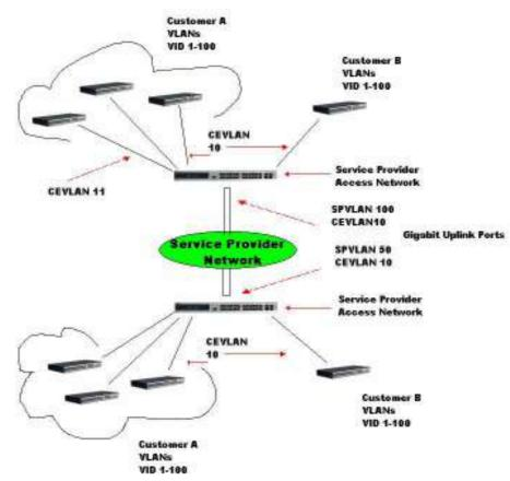
Figure 7-9. Double VLAN Example
