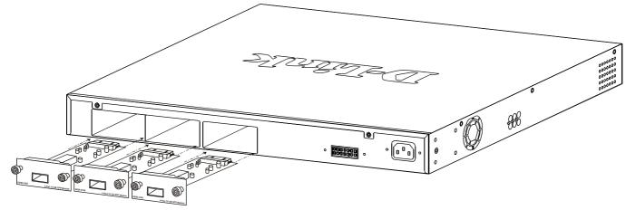
Figure 1-18. Inserting the optional modules into the Switch.
