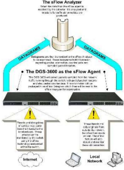
Figure 6-53. sFlow Basic Setup
