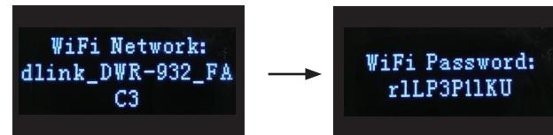
When connecting to the DWR-932 the SSID will be displayed in your device's wireless networking utility. By selecting SSID and entering in the SSID password you will be able to connect to the DWR-932. Please refer to the table below explaining the different screen modes.
