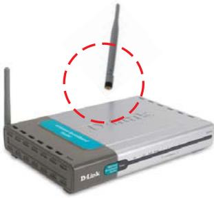
Remove one default antenna from the wireless device and start to assemble!
