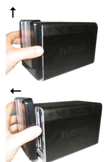
3. Insert a 3.5" SATA hard drive into each available drive bay. Make sure to align the drive connectors to the SATA connectors on the bottom edge inside the drive bay of the DNS-323. Gently push the drive in until it connects. When a drive is inserted properly, you will feel it "seat" into the connector. Some hard drives that are thin or oddly shaped may need to be guided carefully into position. If a drive is not properly seated, the light will not illuminate after powering on the device.
