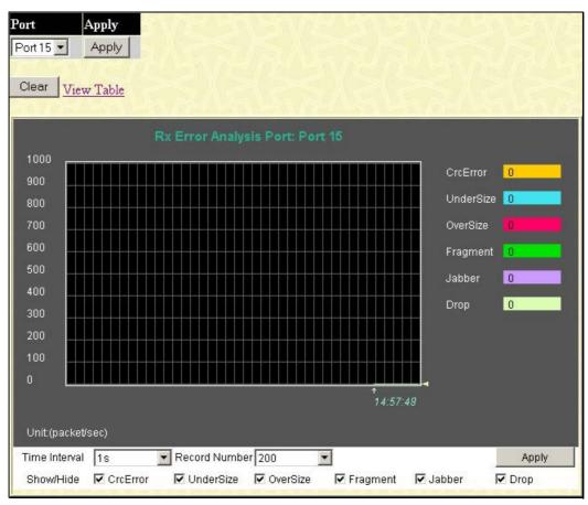
Figure 10-8. Rx Error Analysis window (line graph)
