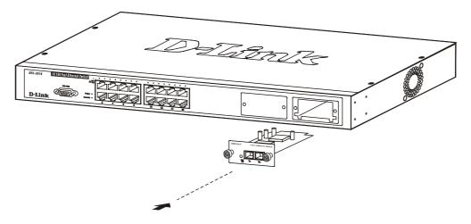
Figure 2-9. Inserting the optional module into the Switch.
