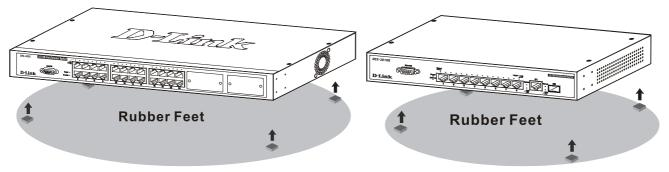
Figure 2-1. Prepare Switch for installation on a desktop or shelf
