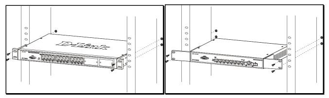
Figure 2- 3. Installing Switch in a rack
