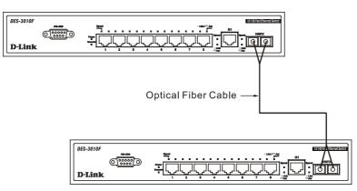
Figure 3- 3. Switch connected to switch using fiber-optic cabling
