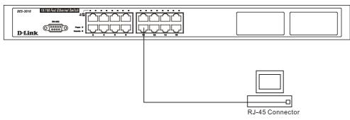
Figure 3-1. Switch connected to an end node
