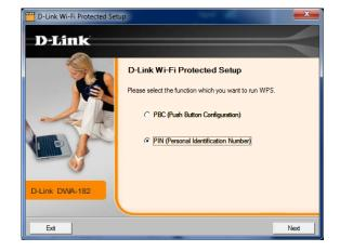
Make sure your access point or wireless router is close by. Write down the number on the screen. Enter this number in your access point or wireless router. Please refer to the manufacture's manual for instructions.
