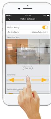
**Sensitivity** - You can adjust the motion detection sensitivity by sliding the marker along the scale.
