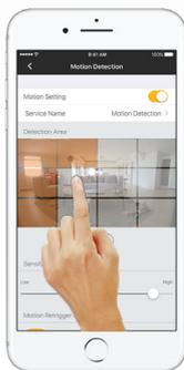
**Detection Area** - Tap the areas of the grid to turn motion detection on or off for that area. Orange shading indicates that an area is being monitored for motion detection.
