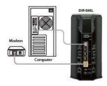
**Step 4:** Plug in the power for your cable or DSL broadband modem and wait for two minutes while the modem initializes.
