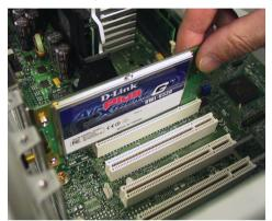
To avoid damage caused by static electricity, make sure to properly ground yourself by first touching a metal part of your computer to discharge any static electricity before working with the DWL-G520 Wireless PCI Adapter.
