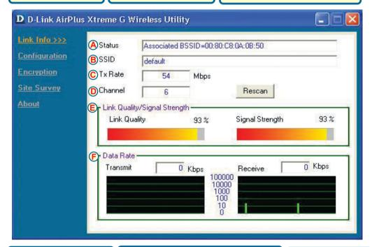
D. Channel: Displays the channel information. By default, the channel is set to 6. Please note that the DWL-G520 will automatically adjust channel depending on the Access Point.
