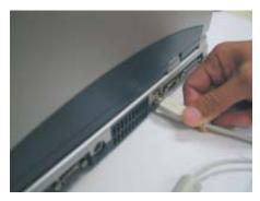
B. Install the DWL-120, firmly insert one end of the USB cable (larger plug) into your computer's USB Port.
