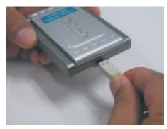
C. Firmly insert the other end of the USB cable (smaller plug) into the DWL-120.
