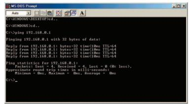
Go to **Start** > **Run** > type **command**. A window similar to this will appear. Type **ping xxx.xxx.xxx** where **xxx** is the **IP address** of the wireless router or access point. A good wireless connection will show four replies from the wireless router or access point, as shown.
