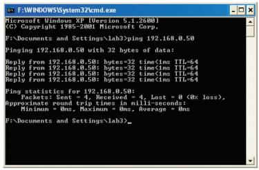
Go to **Start** > **Run** > type **cmd**. A window similar to this one will appear. Type **ping xxx.xxx.xxx**, where **xxx** is the **IP address** of the wireless router or access point. A good wireless connection will show four replies from the wireless router or access point, as shown.
