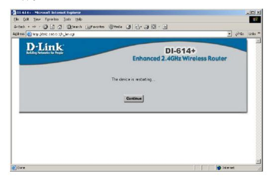
After the DI-614+ has completed its boot up, you will need to release and renew your PC IP address.
