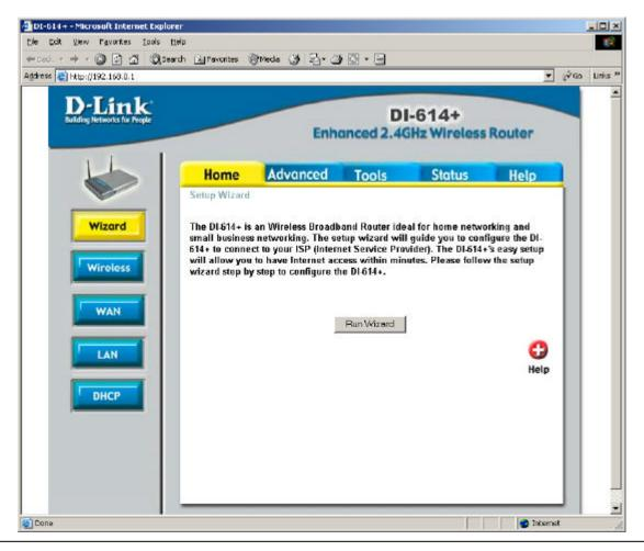
Due to the DSL-300G+ also having the same default IP address, you have to change the IP address of the DI-614+. In this example, its been changed to 10.0.0.1. The DHCP server range will change to this new network automatically.
