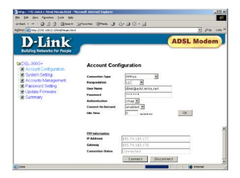
The Through DCHP, the PC IP address would have also changed from 192.168.0.2, to PPP IP address in above screen.
