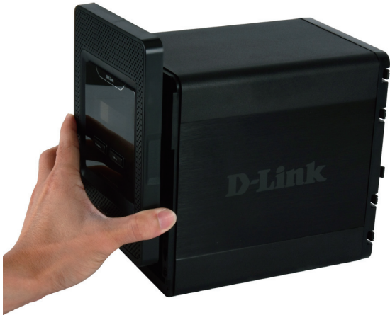
Detach the front cover of the NAS
