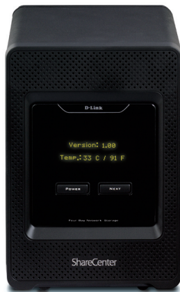
This displays the firmware version and the temperature in Celsius and Fahrenheit.
