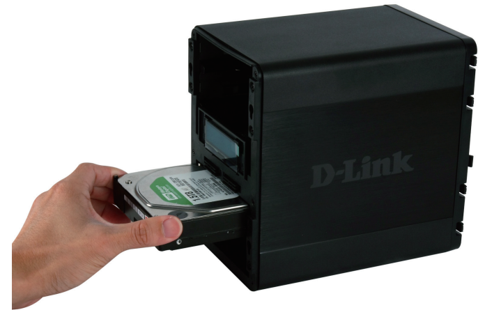
Insert more drives to accommodate RAID 5
