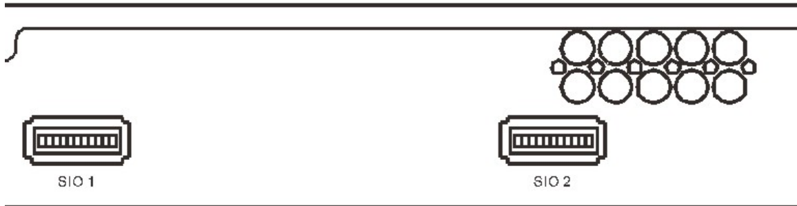
Figure 3- 5. SIO 1 and SIO 2 Stacking ports at the rear of the DGS-3324SR
