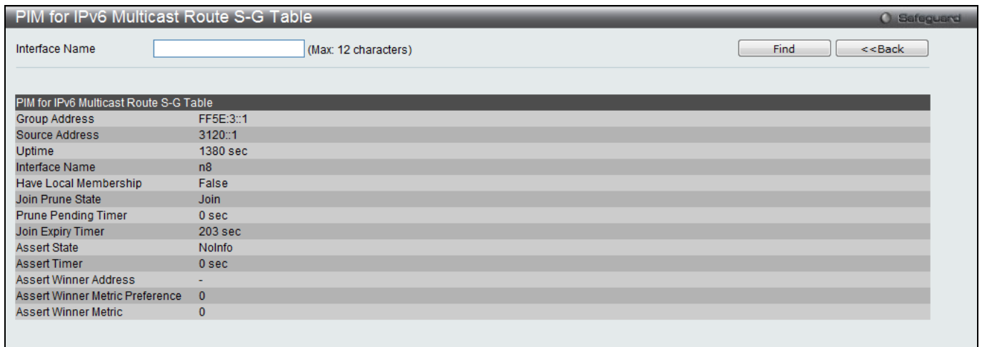
Figure 5-133 PIM for IPv6 Multicast Route S-G Table- View Detail window
