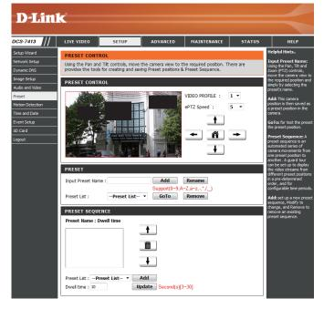
Preset List: To add a preset to the sequence, select it from the drop-down box at the bottom of this window, set the **Dwell** time to determine how long the camera view will stay at that preset, then click the **Add** button. The preset name will appear in the list, followed by the dwell time to view that preset for.
