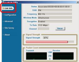
**Status:** Displays the MAC Address of the Access Point that is associated with the DWL-510.
