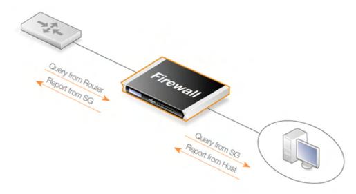
In Snoop mode, the router will act transparently between the hosts and another IGMP router. It will not send any IGMP Queries. It will only forward queries and reports between the other router and the hosts. In Proxy mode, the router will act as an IGMP router towards the clients and actively send queries. Towards the upstream router, it will be acting as a normal host, subscribing to multicast groups on behalf of its clients.
