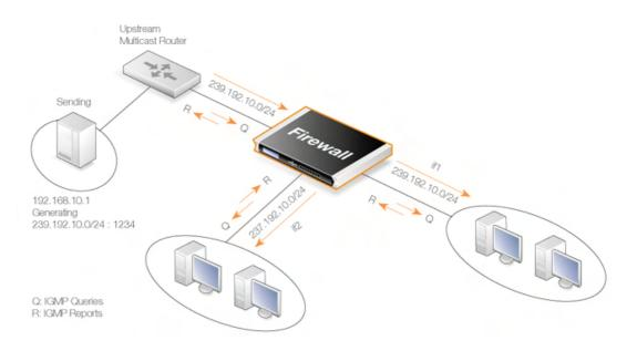
This scenario is based on the previous scenario but now we are going to translate the multicast group. When the multicast streams **239.192.10.0/24** are forwarded through the if2 interface, the multicast groups should be translated into **237.192.10.0/24**. No address translation should be made when forwarding through interface if1. The configuration of the corresponding IGMP rules can be found below in Section 4.5.3.2, "IGMP Rules Configuration - Address Translation".
