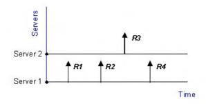
If Connection Rate is applied instead, R1 and R2 will be sent to the same server because of stickiness, but the subsequent requests R3 and R4 will be routed to another server since the number of new connections on each server within the Window Time span is counted in for the distribution.
