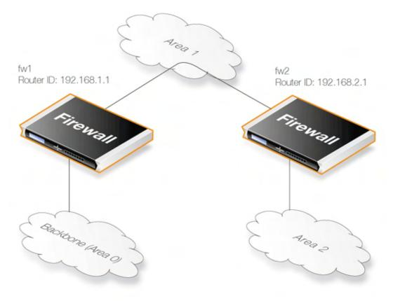
In the above example, the Virtual Link is configured between fw1 and fw2 on Area 1, as it is used as the transit area. In this configuration only the Router ID has to be configured. The diagram shows that fw2 needs to have a Virtual Link to fw1 with Router ID 192.168.1.1 and vice versa. These Virtual Links need to be configured in Area 1.
