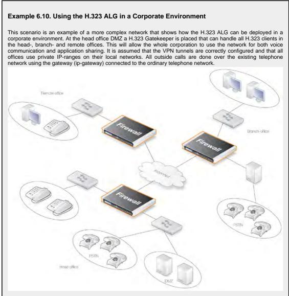
The head office has placed a H.323 Gatekeeper in the DMZ of the corporate D-Link Firewall. This firewall should be configured as follows:
