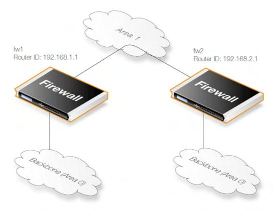
The Virtual Link is configured between fw1 and fw2 on Area 1, as it is used as the transit area. In the configuration only the Router ID have to be configured, as in the example above show fw2 need to have a Virtual Link to fw1 with the Router ID 192.168.1.1 and vice versa. These VLinks need to be configured in Area 1.
