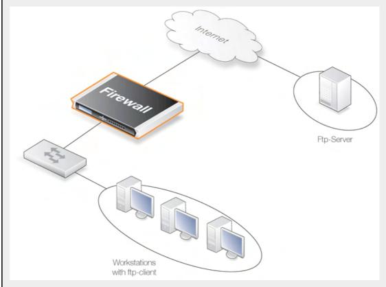
To make it possible to connect to these servers from the internal network using the FTP ALG, the FTP ALG and rules should be configured as follows:
