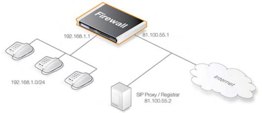
The SIP proxy in the above diagram could alternatively be located remotely across the Internet. The SIP proxy server should be configured with the feature **Record-Route Enabled** to insure all SIP traffic to and from the office peers will be sent through the SIP Proxy. This is recommended since the attack surface is minimized by allowing only SIP signalling from the SIP Proxy to enter the local network. The steps to follow are:
