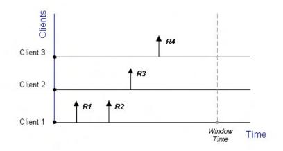
When the Round Robin algorithm is used, the first arriving requests R1 and R2 from Client 1 are both assigned to one sever, say Server 1, according to stickiness. The next request R3 from Client 2 is then routed to Server 2. When R4 from Client 3 arrives, Server 1 gets back its turn again and will be assigned with R4.
